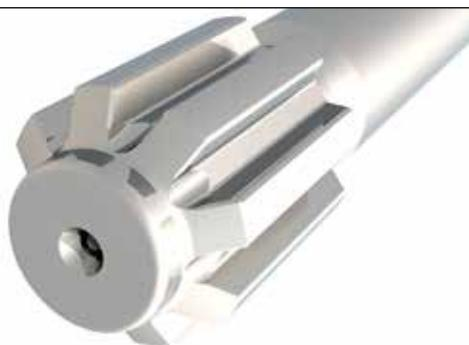
Hydraulic shanks generally have at least a 5 to 14-spline configuration. Pneumatic shanks tend to have internal or through-flushing. They can be identified by their lugs or 4-spline configuration.
