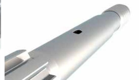
Shank adapters with external flushing can be identified by machined slots in the center of the adapter. The slots are positioned between seals inside the flushing housing / head of the rock drill.
