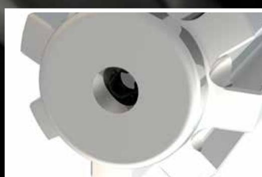
Internal flushing shank adapters use a water tube inside the rock drill. The tube fits into the end of the shank adapter and is sealed with an O-ring. This allows the water to transfer from the rock drill to shank adapter, which in turn allows it to flow through the rest of the drill string.
